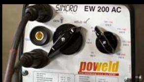
AC engine driven welders are especially developed for light construction work. After welding you can change the switch to generator-mode and use full 6kVA single phase 230V power for drilling and grinding. Available in gasoline and diesel versions.
