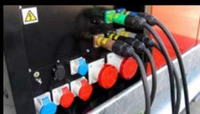
All EPSR generating sets are equipped with the socket configurations B15 up to 150kVA and B16 from 180kVA on: see legend in our price list. You never have to search for the right male socket. Besides the sockets you have five 500A 'Powersafe' power connectors.
