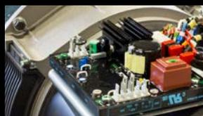
AVR stands for Automatic Voltage Regulator to maintain a constant and stable voltage. This results in better performance for sensitive appliances.
