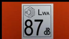
The Kubota range of Europower generating sets can indeed be called "super-silenced". Sound levels vary from 60 to 65dB(A) at 7m or from 85 to 90 LWA. This is comparable with people speaking in a room or with an ordinary vacuum cleaner.
