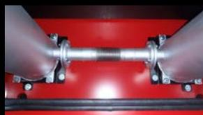
2 independent mufflers, one of which works on resonance and the other on sound absorption.
