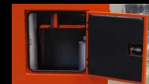
The inspection panel has been replaced by an inspection door for easy access when cleaning the radiator.
